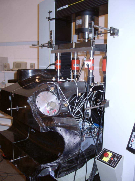
Figure 13 Acoustic Emission Testing of an F1 Monocoque
