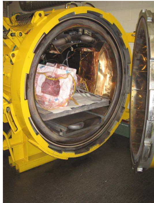
Figure 12 Nosebox loaded into the small autoclave for processing
