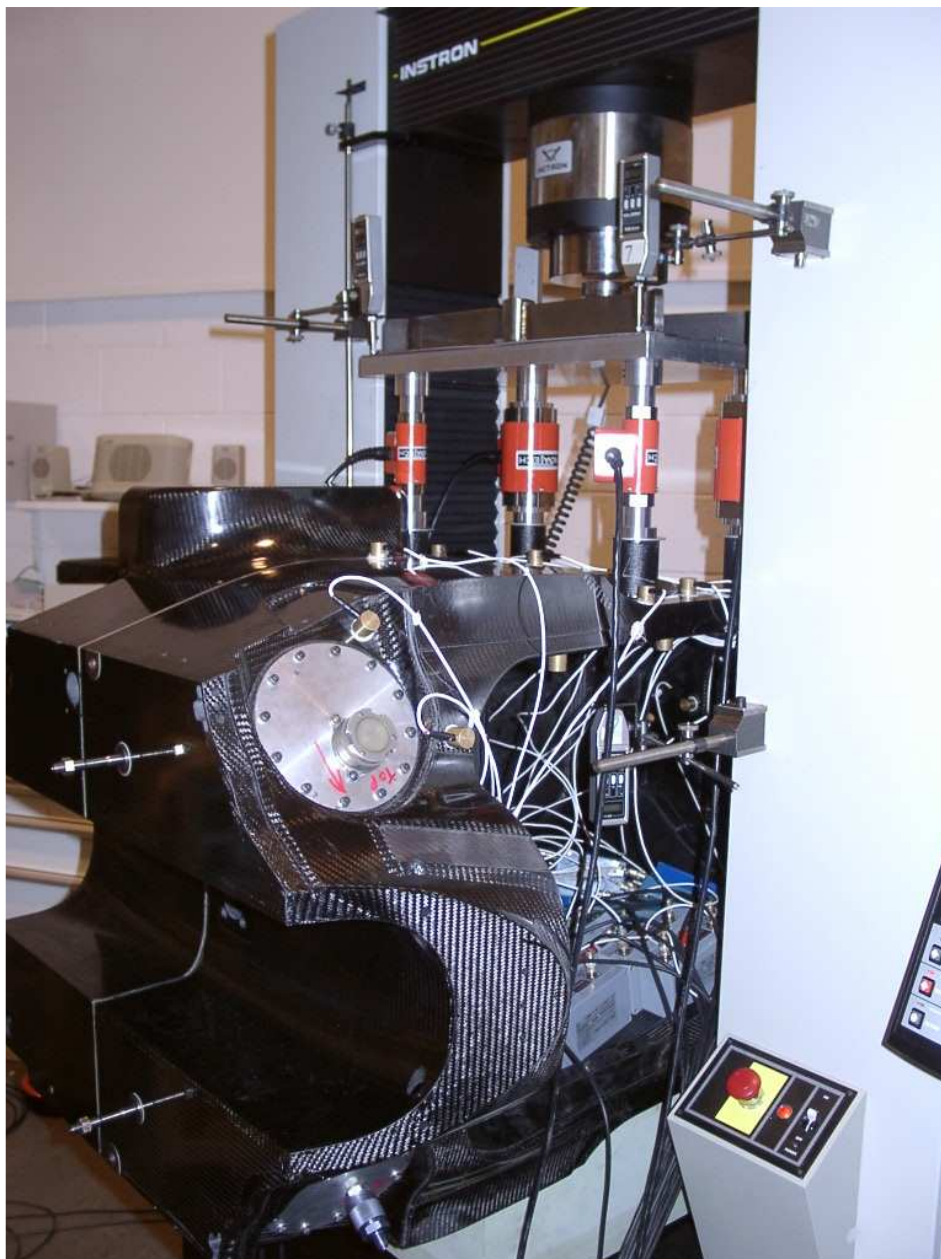
Figure 11 Showing A23 chassis in side static squeeze rig
