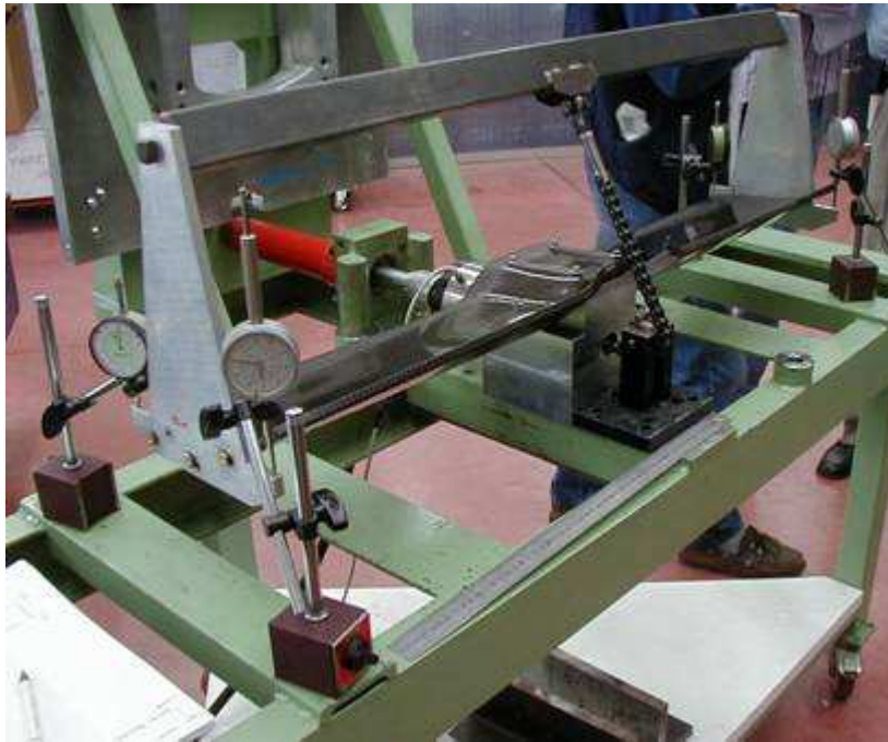
Figure 2 Showing a purpose built proof test rig for a down force wing
